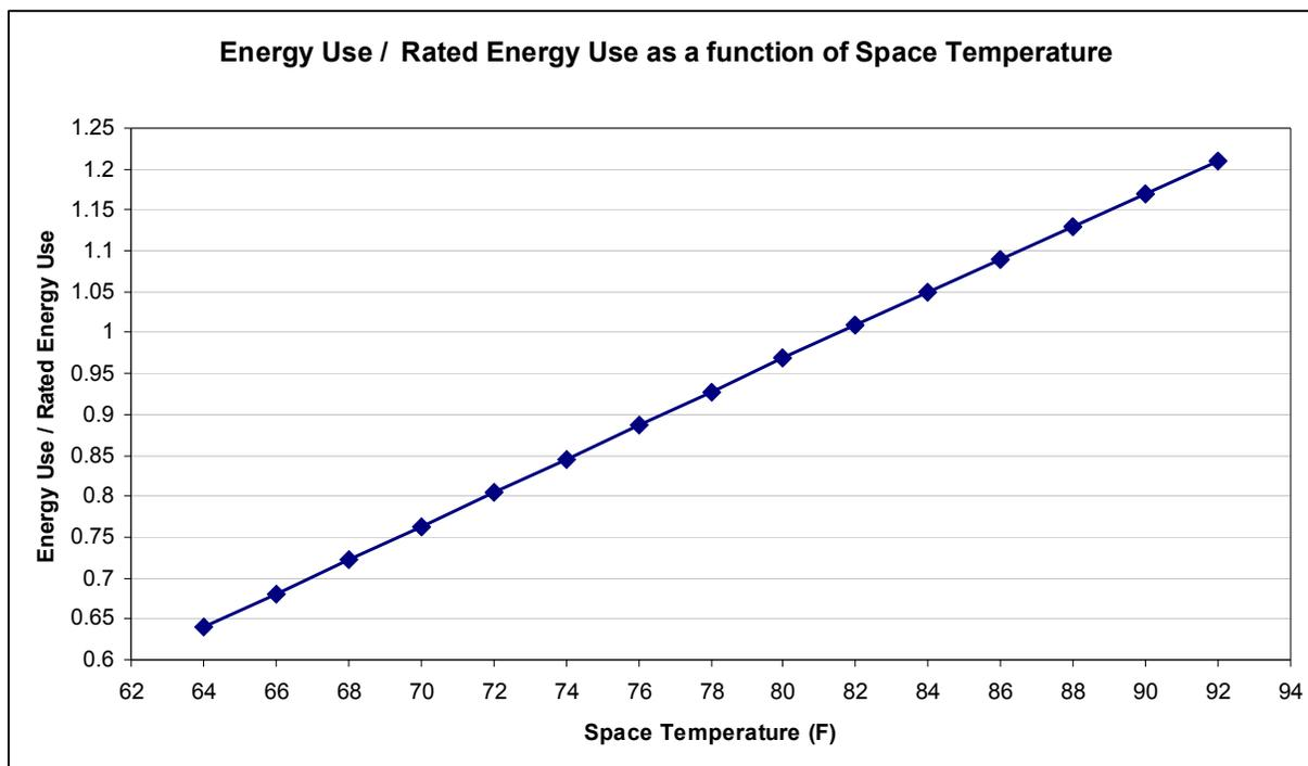
Figure 9: Refrigerator Energy Use as a function of Environmental Temperature
