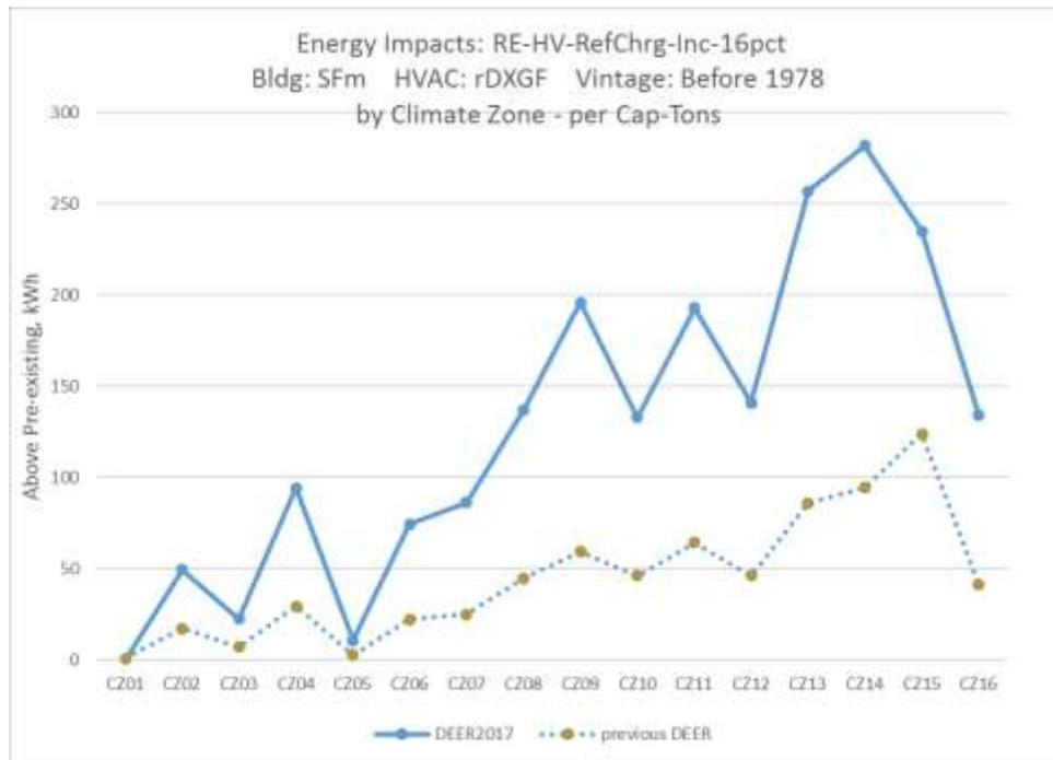
Figure 16. Example energy impacts for a high increase in refrigerant charge – Single Family, pre-1978 Vintage
