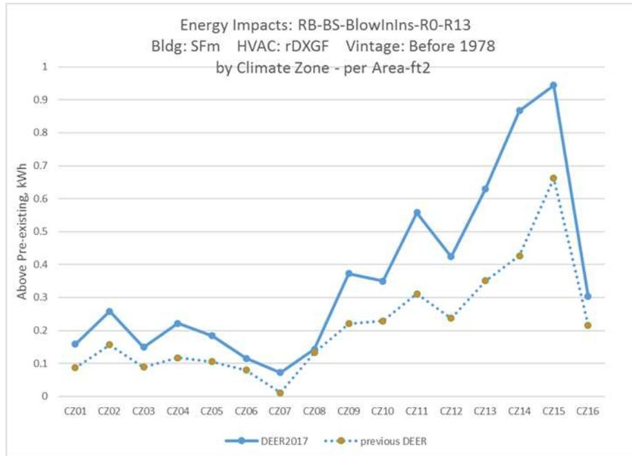
Figure 10. Example of energy impact changes in a residential wall insulation measure
