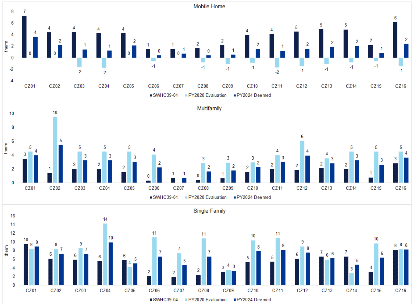
Figure 2-3. Deemed and Evaluated Gas Savings for Direct Install Delivery of SWHC39-04 Smart Thermostat
