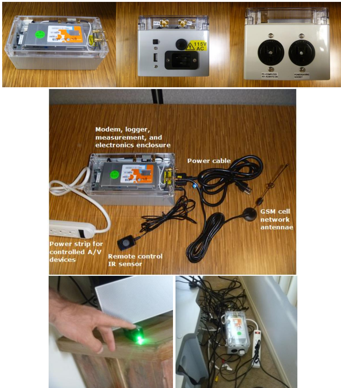
FIGURE 9 - A/V APS INSTRUMENTATION, LED LIGHT, AND INSTALLED INSTRUMENTATION
