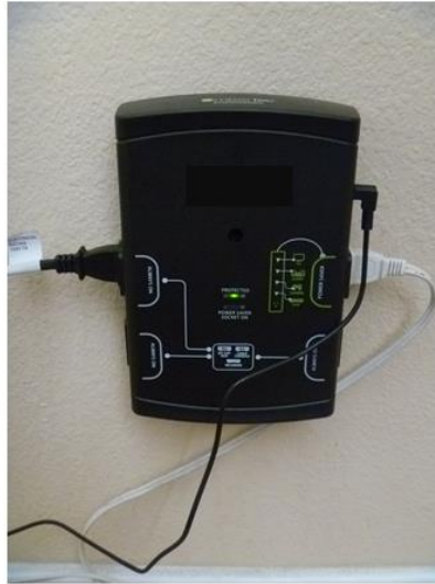
FIGURE 11 - INSTALLED A/V APS DEVICE AFTER REMOVAL OF INSTRUMENTATION
