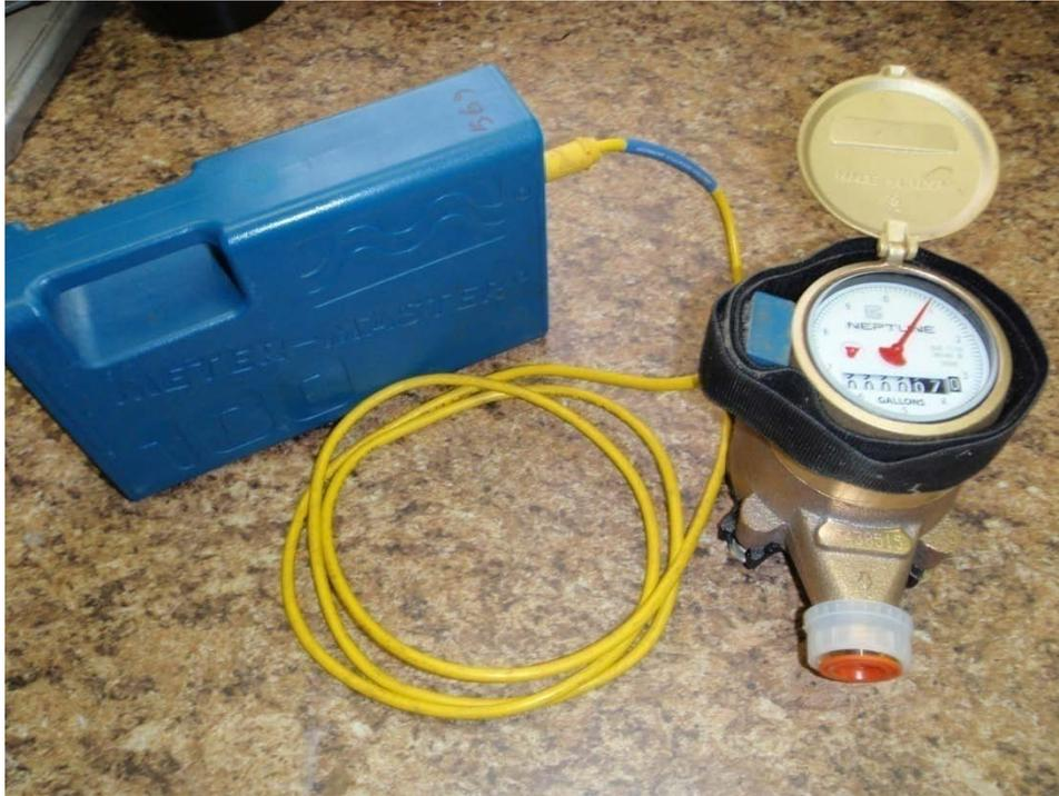
**Figure E-2: Meter Master 100 Flow Recorder Attached to Commercial Water Meter**
