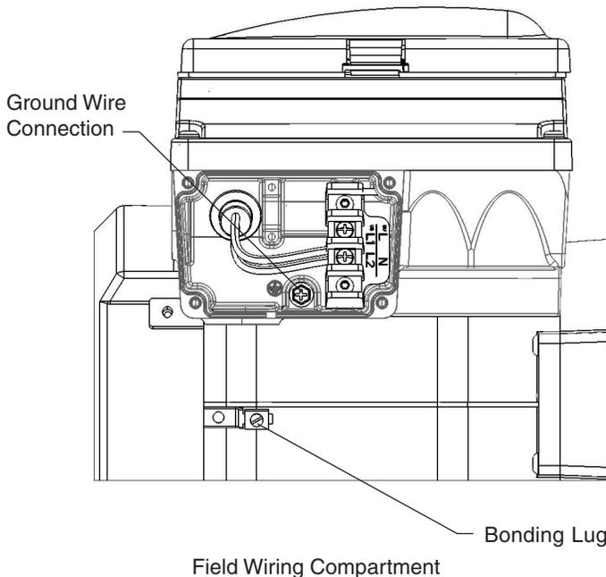
**Note:** When the pump is started and stopped by removing power with a relay or timer, a two-pole device should be used to apply and remove power to both POWER LINE TERMINALS.
