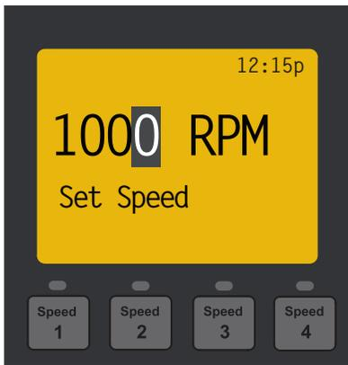
Setting the Anti Freeze Pump Speed
