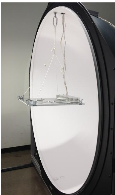
FIGURE 1 TROFFER SETUP IN INTEGRATING SPHERE
