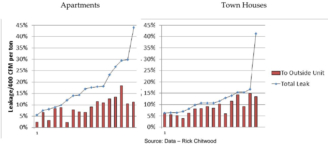
In summer, the effects of duct leakage include capacity loss from supply leaks, infusion of superheated attic air from return leaks, and house infiltration due to the imbalance between supply and return leakage. The infiltration effect occurs regardless of whether the dominant leakage is in the supply system or the return system. The leakage imbalance was estimated by the “Half Nelson” test combined with the operating pressures of the system. The calculation occurs in the following manner:
