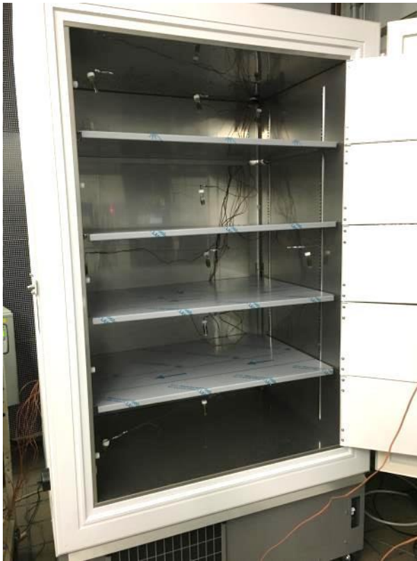
FIGURE 7: FIVE COMPARTMENT FREEZER VIAL PLACEMENT
