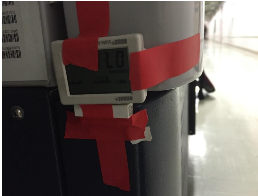
FIGURE 8: DOOR SENSOR PLACEMENT
