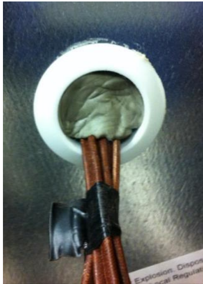
FIGURE 5: THERMOCOUPLE ROUTING
