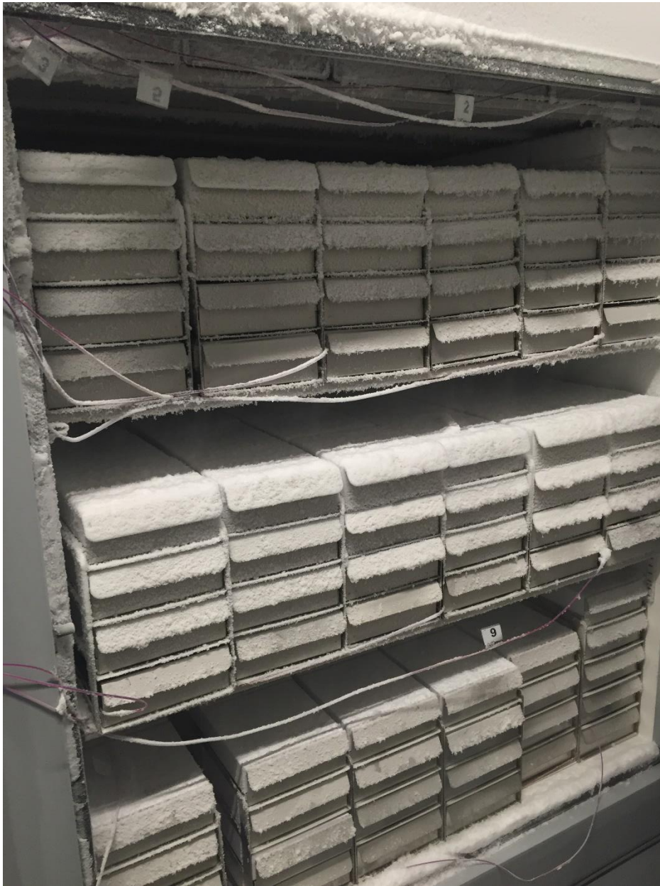
FIGURE 14: THERMOCOUPLE PLACEMENT IN FULL ULT FREEZER
