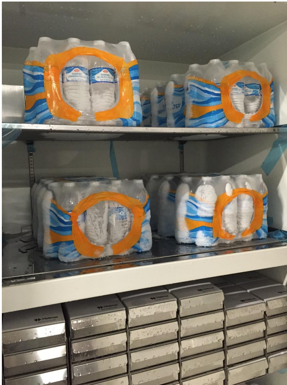
FIGURE 15: ULT FREEZER FILLED WITH WATER
