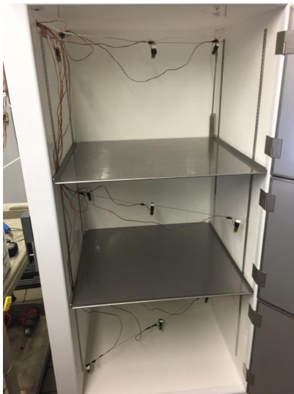
FIGURE 6: THREE COMPARTMENT FREEZER VIAL PLACEMENT
